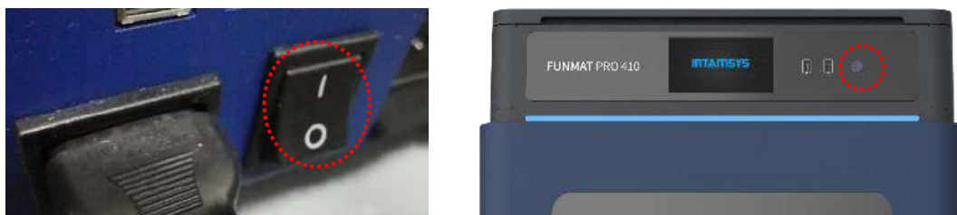
Figure 2.4 Power switch and startup button
