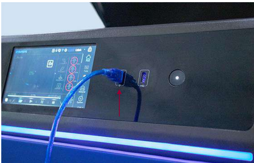
Figure 5. 18 Connection method of USB print mode
