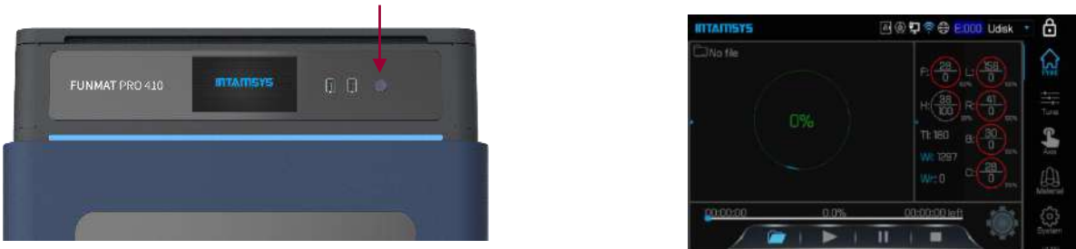
Figure 5. 2 ON/OFF Switch and startup interface
