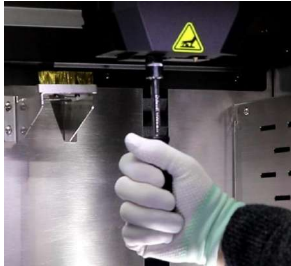
Figure 5. 9 Replacement of nozzle
