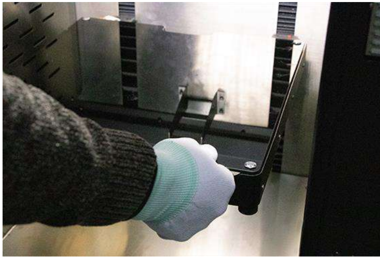
Figure 5. 11 Installation of printing buildplate glass
